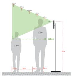
Recommended Installation Height: 150cm Temperature Measurement Distance: 30cm to 120cm
